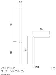
Joint pin Corner joint pin
