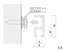
●推奨荷重:取付ピッチ300㎜以内/8kg Recommended load : Installation pitch needs to be within 300mm / 8kg
